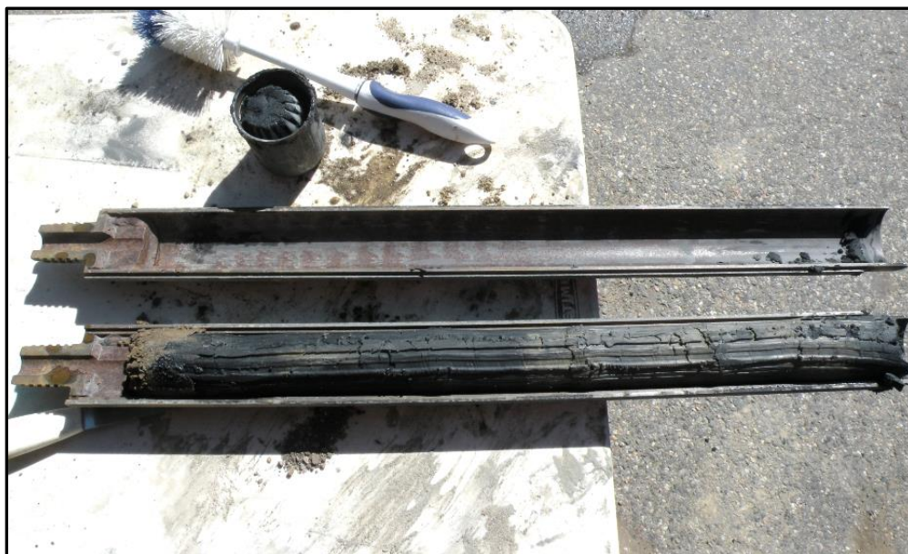
Drill core of subsurface soil collected from a soil boring illustrating petroleum-contaminated soil. The left half of core sample (black) has a heavy petroleum stain, and the right half (gray) has a lighter petroleum stain.
