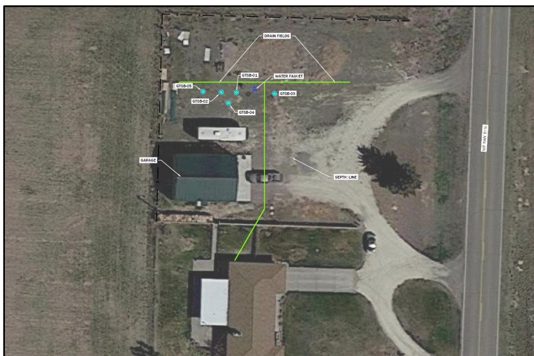
Photo: Aerial view of the former Garth Taylor Facility showing the location of the soil borings (teal-colored dots) installed during the 2019 remedial investigation in the former underground storage tank area.
